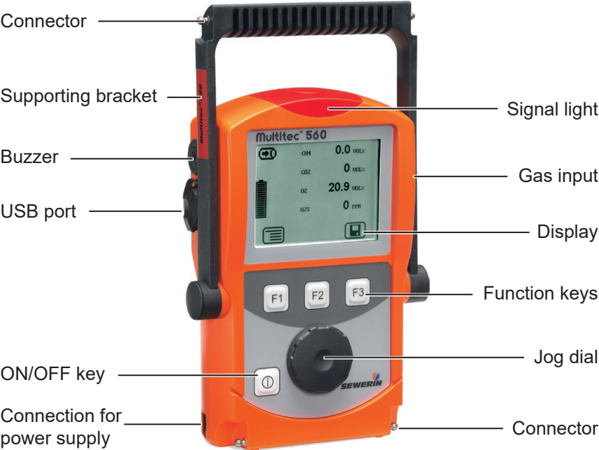
Fig. 1: Multitec 560 device overview
