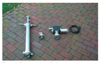
Picture 11: Stopper, stand pipe, flushing adapter
