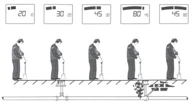
Picture 4: Acoustic leak detection
